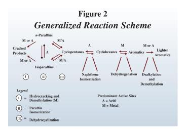
UOP has made great advances over the past two decades combining improved catalyst formulations with lower operating pressures that improve yields in the key reactions. Catalyst system performance, as measured by activity and selectivity to desired reactions, is achieved by the balance between acid and metal sites.
