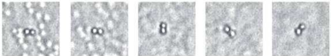
Figure 7.8: A group of four 1 \mu\text{m} diameter silica spheres that is tweezed and lifted vertically whilst simultaneously being rotated through the sample cell. The interference pattern used is an (l = 1) + (l = -1) pattern of two spots. Only the top two spheres are visible as the structure is viewed from above.
