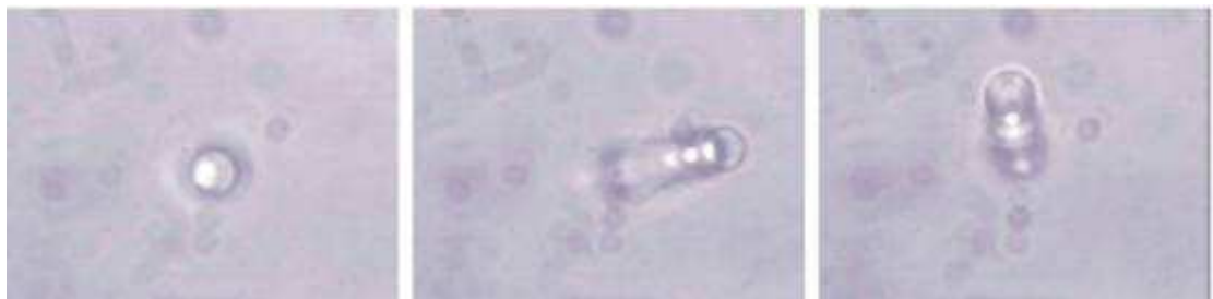
Figure 3.7: Tilting of a stack of six 5 \mu\text{m} spheres as the laser beam is inclined, viewed from below in an inverted geometry.
