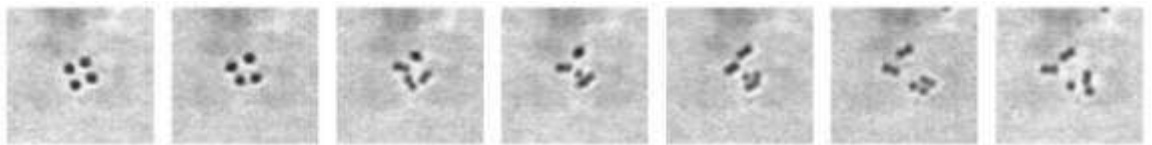
Figure 7.10: The same cubic structure is seen to collapse, revealing the eight constituent spheres as the trapping laser beam is blocked.
