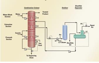
In the caustic regeneration section, the mercaptan rich caustic solution, containing Merox WS catalyst, is injected with air and the mixture flows into the oxidizer
