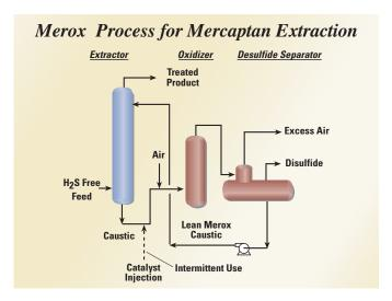
The mercaptan rich caustic solution containing Merox WS catalyst is injected with air and the mixture flows into the oxidizer where the dissolved mercaptans are catalytically oxidized to water insoluble disulfide oil.
