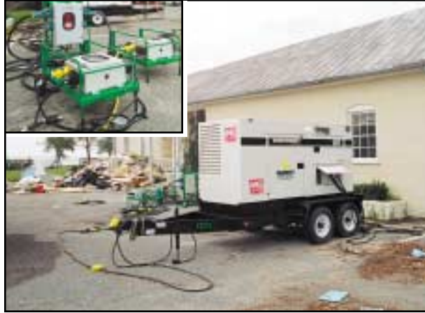
Above: A 100-kW diesel generator and distribution equipment used by Cary Reconstruction Co. at a water-damaged, historic building in Edenton, NC Below: Six dehumidifiers were rented from Sunbelt to dry out Fred Moody & Sons Garage in Kinston, NC. Isabel ripped off part of the roof.
