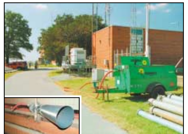
Above: A 375-cfm diesel air compressor rented by Garner Environmental Services to power venturi air horns providing ventilation inside the flooded Midtown Tunnel in Norfolk Below: One of two 6" Quiet Flow™ pumps utilized by Garner Environmental inside the Midtown Tunnel
