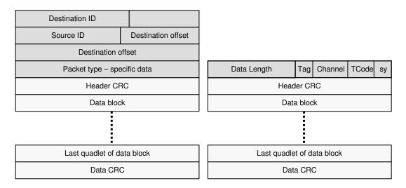
Figure 4- Asynchronous and Isochronous packets.
