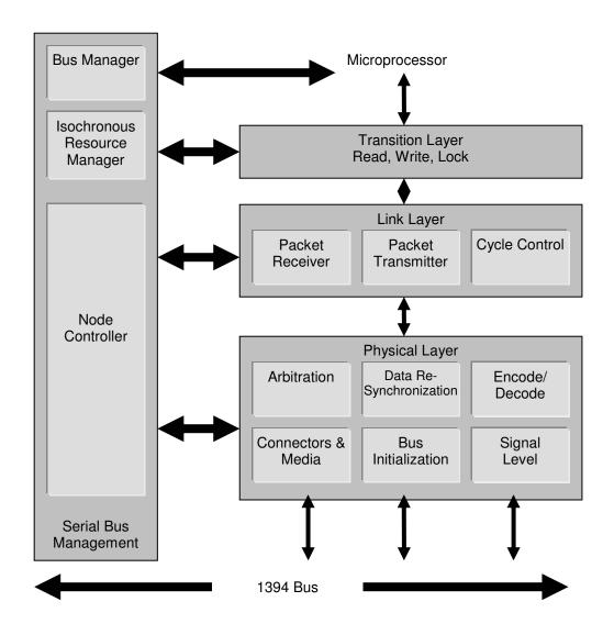
Figure 3 - The 1394 Protocol Stack and Serial bus Management Controller
