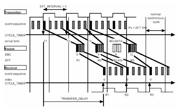
Figure 6 - Blocking and Packetization
