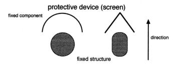
A protective screen shall be defined as a fixed component that serves as a windscreen or windbreak designed to protect another fixed element of the bicycle in order to reduce its wind resistance.
