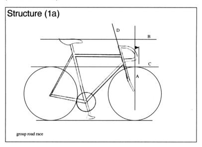
1.3.023 For road time trial competitions and for the following track competitions: individual and team pursuit, kilometre and 500 m, an extension may be added to the steering system. The distance between the vertical line passing through the bottom bracket axle and the extremity of the handlebar may not exceed 75 cm, with the other limits set in article 1.3.022 (B,C,D) remaining unchanged. A support for the elbows or forearms is permitted (see diagram «Structure (1B)»).
