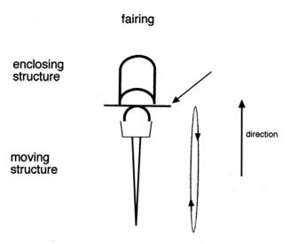
practical way of confirming the existence of fairing on a moving part such as a wheel: it should be possible to pass a rigid card (like a credit card) between the fixed structure and the moving part.
