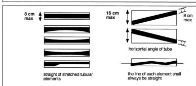
**1.3.021** For road time trials and for track competitions, the elements of the bicycle frame may be tubular or solid, assembled or cast in a single piece in any form (including arches, cradles, beams or any other). These elements, including the bottom bracket shell, shall fit within a template of the «triangular form» defined in article 1.3.020. (See diagram «Shape (2)»).
