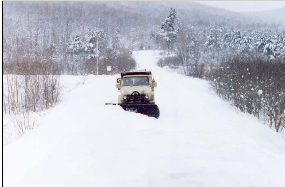
Figure 5. The SEE tractor is the most versatile snowplow in the U.S. Army inventory. It can plow off-road as easily as it plows paved and unpaved roads, staging areas, storage sites, or any other requirement. Such work requires that the SEE be maintained daily and be fully operational at all times.
