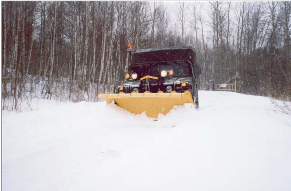
Figure 11. The HMMWV snowplow has proven to be an effective attachment and is in service in Europe and in the Far East as well as in CONUS. It is an 8-foot, hydraulically operated plow capable of plowing MSRs and various classes of roads and highways. For safety purposes, the maximum allowable speed while snowplowing is 10 mph.
