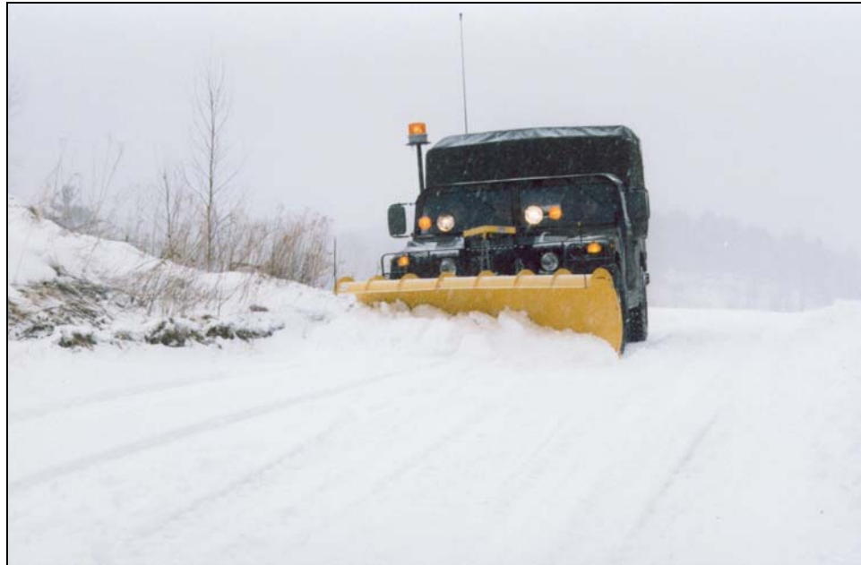
Figure 9. HMMWV with 9-foot plow, clearing snow from an access road. The early snowplows were 9 feet wide and worked very well; however, to improve safety, since 2000, all HMMWV plows are 8 feet wide. This plow is fully reversible and has an automatic trip-edge.
