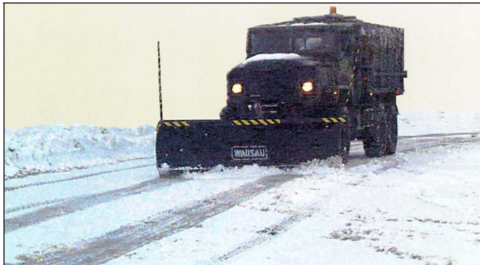
Figure 18. 5-ton truck with snowplow “cleaning up” after a major storm. The use of plow guides is an absolute must for a plow of this size.
