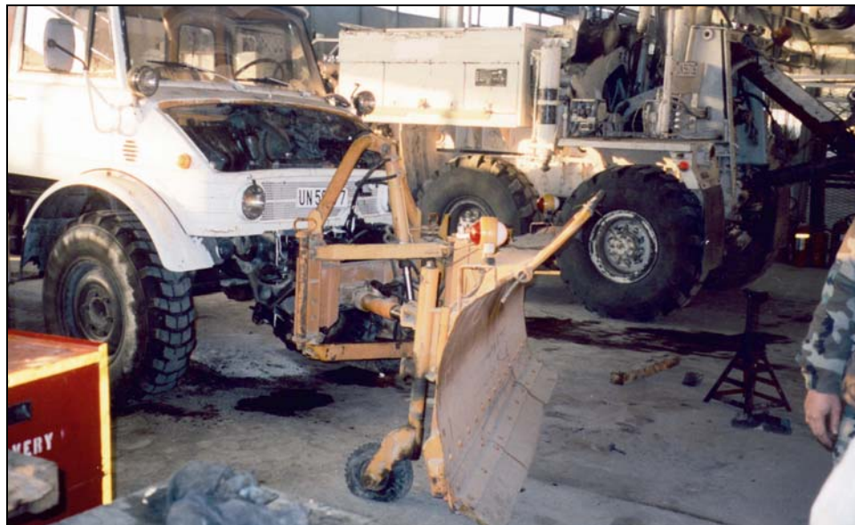
Figure 4. Fifty-year-old Schmidt (of Germany) snowplow mounted on a Unimog tractor. This snowplow provided quality service at Baumholder, Germany, for 43 years before being shipped to Macedonia. This fully reversible segmented snowplow with fully operational trip-edges still works well today. The Unimog is a sister vehicle to the SEE tractor that was manufactured in the United States by Freightliner Corporation.
