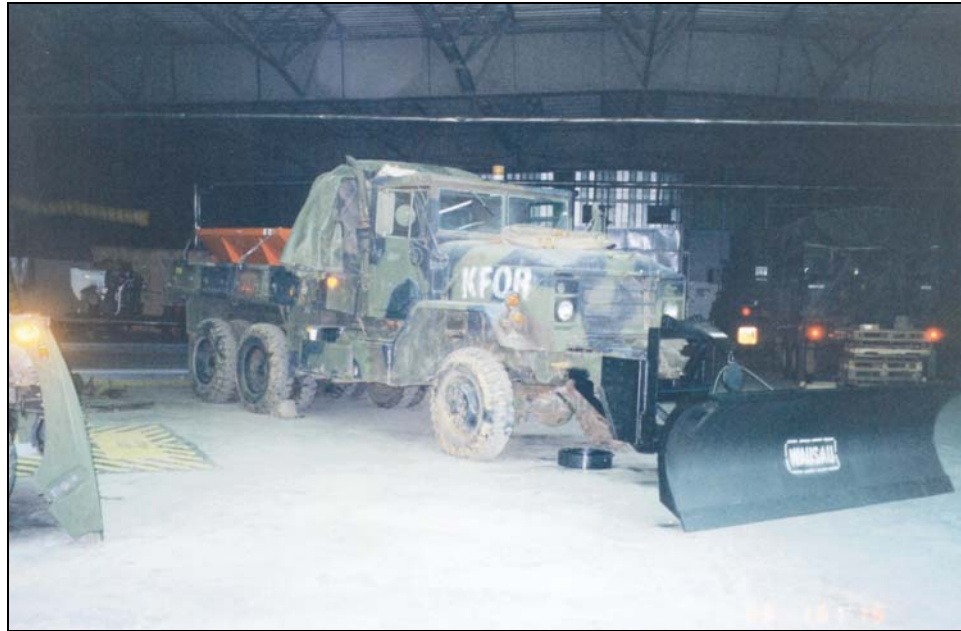
Figure 16. Wausau-brand snowplow manufactured by Schmidt Engineering and Equipment, Inc., of New Berlin, Wisconsin, mounted on a 5-ton truck. The truck has a Henderson “Chief” spreader mounted in the truck bed. Both items can be used simultaneously or separately.
