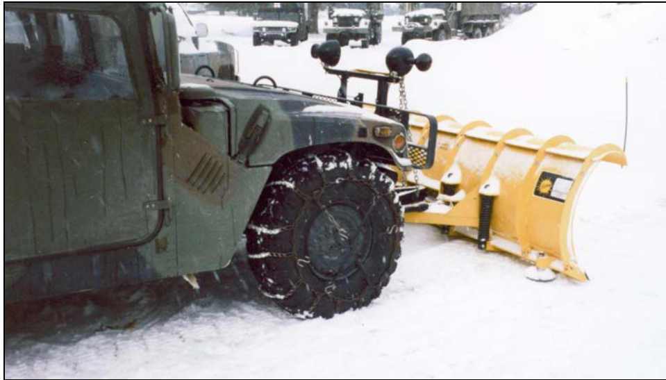
Figure 8. HMMWV snowplow mounted on a HMMWV with chains on all four wheels. This snowplow can be mounted and dismounted in less than a minute after the on-vehicle frame push-plates and the wiring harness are installed.
