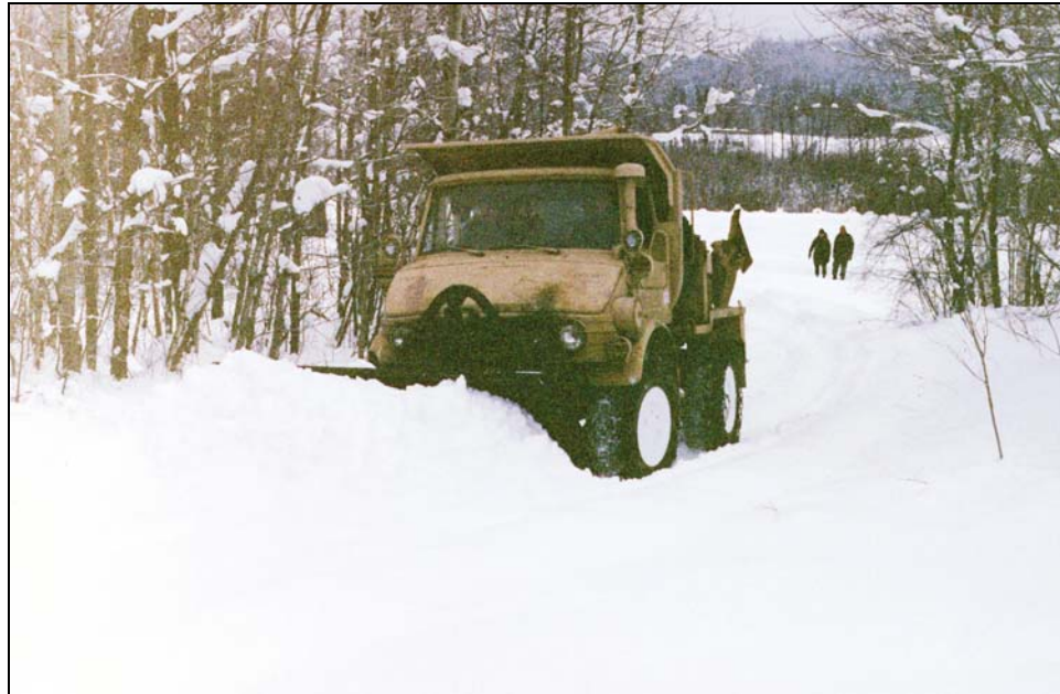
Figure 6. Plowing steep grades uphill is not a problem for the SEE tractor and its 10-foot fully reversible hydraulic plow. Chains are required on all four wheels at all times to ensure traction and as a safety measure. The SEE tractor snowplow can be completely installed on the SEE in less than 30 minutes.
