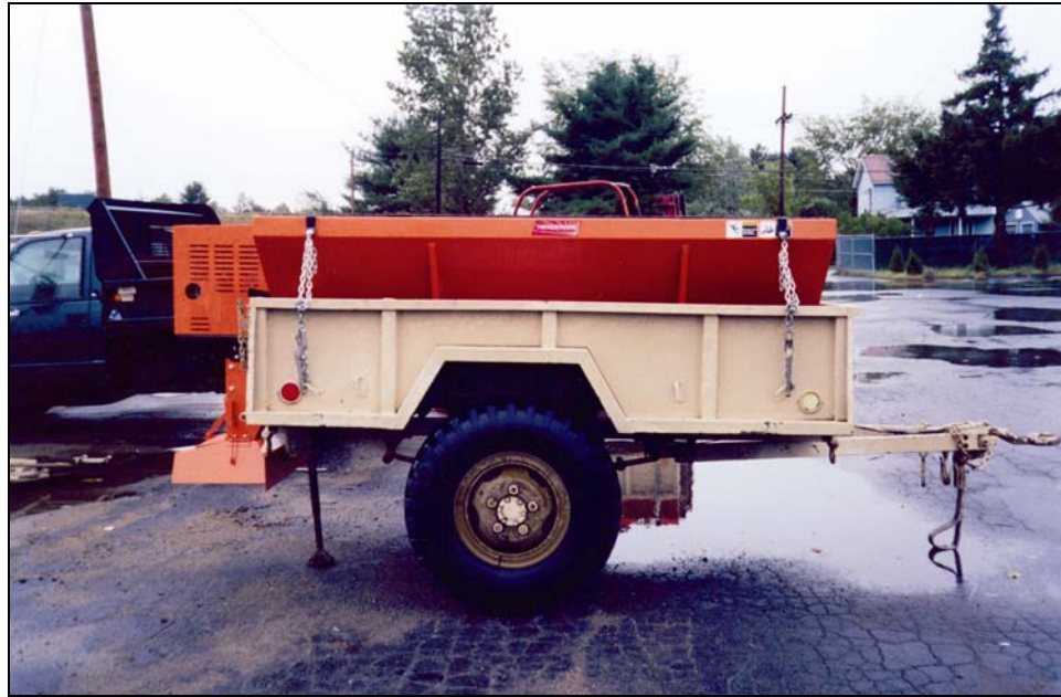
Figure 19. The 6-foot Henderson spreader was mounted on the M100 trailer at the request of commanders in Kosovo. Efforts were made to try to discourage this arrangement because of safety issues. However, the unit insisted, and four of these were made up and shipped. All four suffered accidents—one turned over and took the HMMVW with it. Spreaders should never be mounted in trailers.
