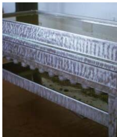
Alla-barese filter showing the oil in the top passing through cotton and dripping into the reservoir below
