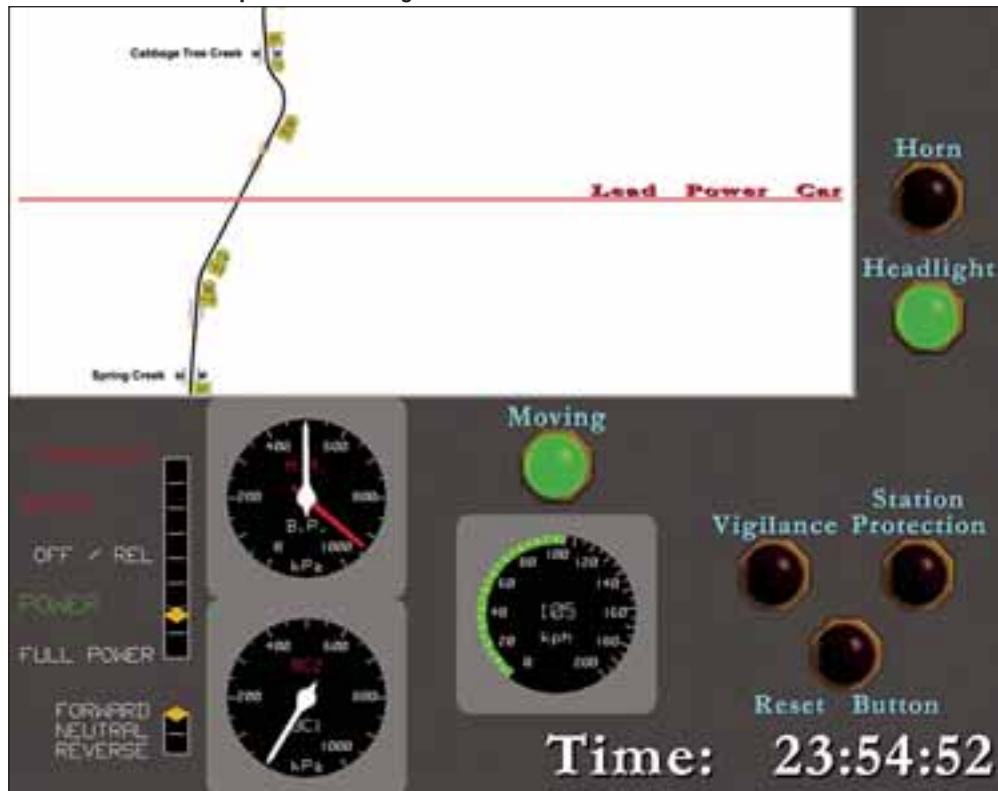
FIGURE 4: Driver feathers power to 60%; train maintains a constant speed of approximately 110 km/h up to and including accident site
