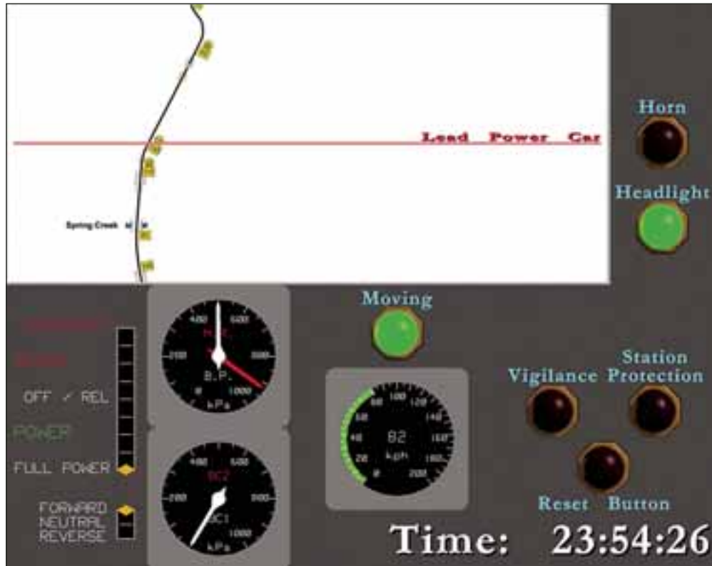
FIGURE 3: Train approx at 417.783 km, location of 150 km/h 'Speed Board'. Train accelerates from 82 km/h under full power
