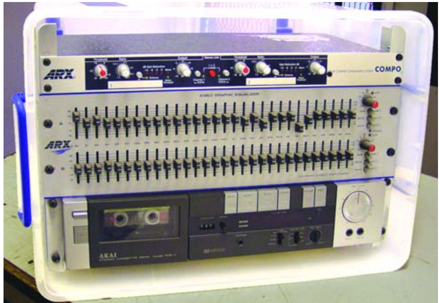
The Fry-conomatic features bended aluminium racks fixed to the plastic case with state-of-the-art pop rivets.
