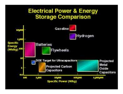
Figure 1- : Plot of energy versus power for various fuels and energy storage devices.
