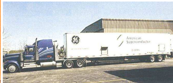
Trailer-mounted D-SMES Unit (3MW and up to 16MVA capacities)
