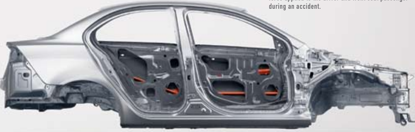
RISE BODY Lancer's safety design and stiffness both come from Mitsubishi's RISE unibody design. The RISE body utilizes high-tensile-strength steel in strategic locations to increase stiffness. It also disperses energy loads during side and rear crash impacts, enhancing occupant protection and helping to protect the fuel system's integrity.
