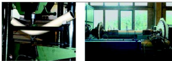
Figure 5 (A & B) Special mechanical testing of RTP. Left: 4" RTP subjected to bending test, no failure at a bending radius of 300 mm. Right: "Flexirig" test bench for simultaneous dynamic tensile, bending, and torsional load testing.
