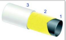
The Soluforce® pipe consists of three layers being a standard PE pipe grade liner pipe (1) reinforced with synthetic fibres (2) and a specially design PE outer protection layer (3). The liner pipe ensures a corrosion resistant fluid tight containment, the reinforcing layer gives the system the ability to take up the high-pressure rating and the outer layer protects the pipe from abrasion and the environment.
