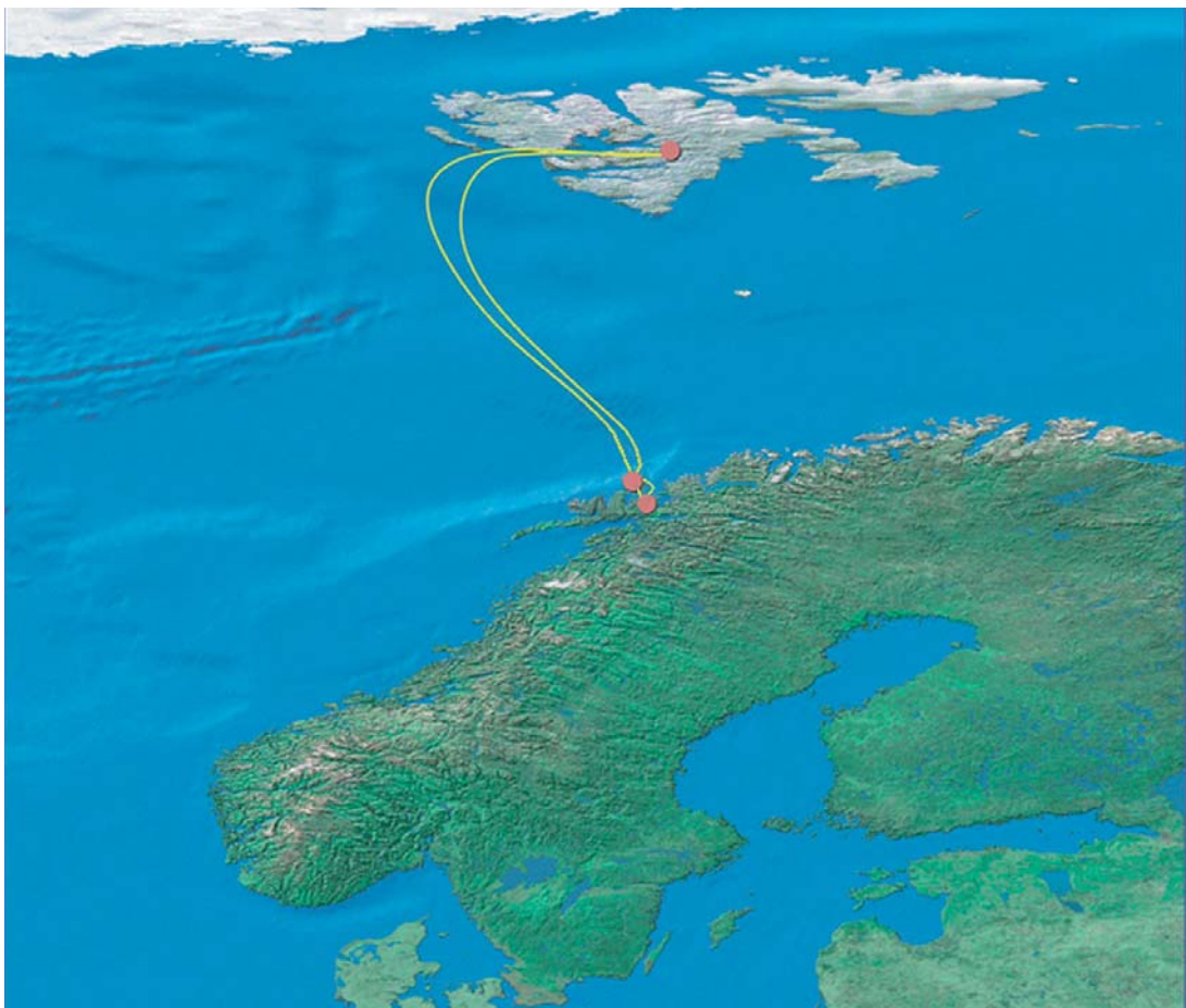
Two independent cables, each with very large capacity, now connect Svalbard with mainland Norway and the international fibre network
