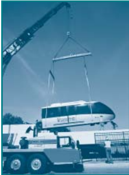
Fabricated in Olten, Switzerland, the four 'nose' vehicles of Clarian's People Mover trains are 28-foot long, six feet longer than the center cars.
