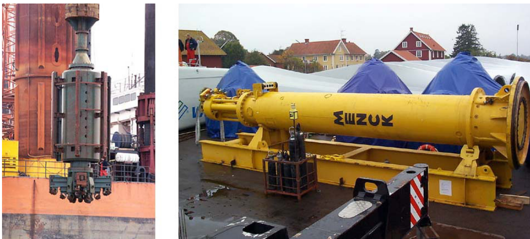
Figure 2.7: Drill (left) and pile-driven (right) monopile installation equipment (Courtesy of www.windpowerphotos.com )
