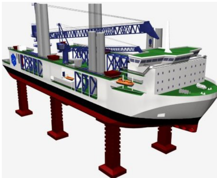
Figure 2.3: Mayflower TIV-1 installation vessel (Courtesy of Mayflower Energy)
