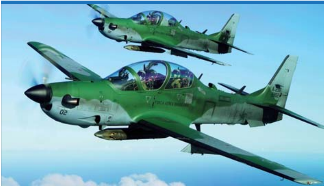
Coin operations may involve turboprop aircraft, such as Embraer Super Tucanos. Brazilian Air Force A-29Bs are shown armed with rocket pods and wing-mounted machine guns. (Embraer)
