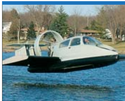
The US Navy plans to evaluate the special operations potential of the Universal Hovercraft UH-19WRX Hoverwing, which is basically a hovercraft with stub wings attached. (Universal Hovercraft)
