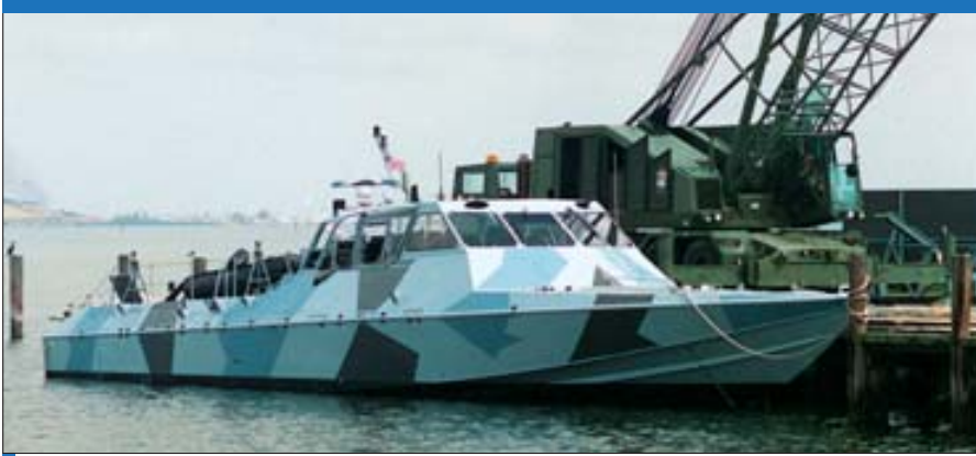
The Mk V special operations craft is one of the most recent additions to the US Navy Seal's equipment list. The boats can travel in excess of 50 knots (93 km/h) and are powered by two Kamewa K50S waterjets. (US Navy)
