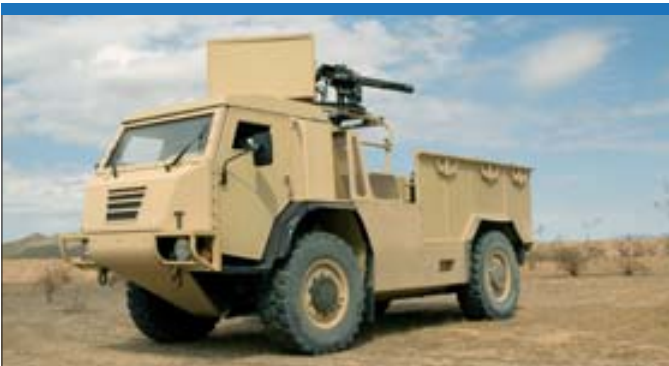
Lockheed Martin has developed a 4 x 4 Armored Proof of Concept Vehicle which could be suited for special forces long-range patrols. Options include armour protection. (Lockheed Martin)
