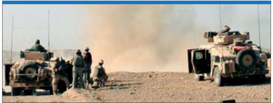
The primary patrol vehicle used by the American land special forces is the AM General Ground Mobility Vehicle that is derived from the High Mobility Multipurpose Wheeled Vehicle. (US Army)
