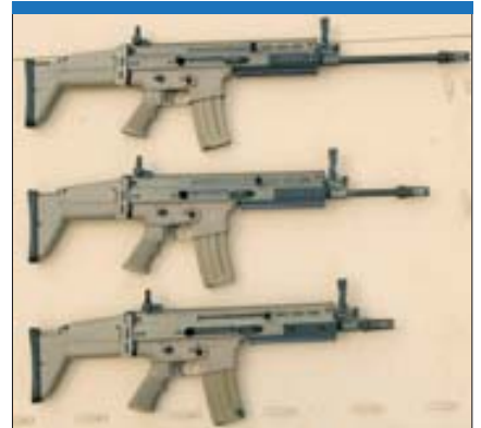
FN Herstal's 7.62 mm Mk 17 Mod 0 Scar-H can be fitted with a close quarter combat (bottom), a standard (centre) or a sharpshooter variant barrel (top). (FN Herstal)
