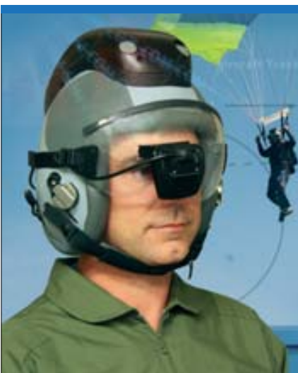
In September 2007 Rockwell Collins unveiled its Paranav GPS-based helmet-mounted navigation system with integral display. Over 100 jump tests have been carried out from up to 28,000 ft. (Rockwell Collins)
