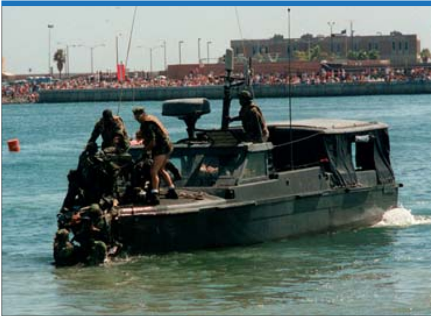
Although no longer in service with the US Marines, the Seafox remains in use with Egypt's naval SOF. The craft is powered by a pair of 6V-92TA diesel engines which develop 520 horsepower. (US Navy)
