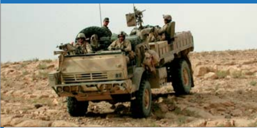
A number of Stewart & Stevenson 2.5-tonne Light Medium Tactical Vehicles have been modified to provide logistical support for long-range patrols. (Stewart & Stevenson)
