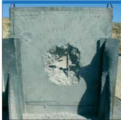
Instalaza is currently developing a new tandem warhead for its C90 and Alcotan 100 ABK. The type for the latter weapon is currently being qualified with the Spanish Ministry of Defence and consists of a precursor warhead able to create a 50 mm diameter hole in 350 mm of concrete to enable the main warhead to penetrate and disperse some 2500 steel balls with a lethal radius of ten metres. (Instalaza)
