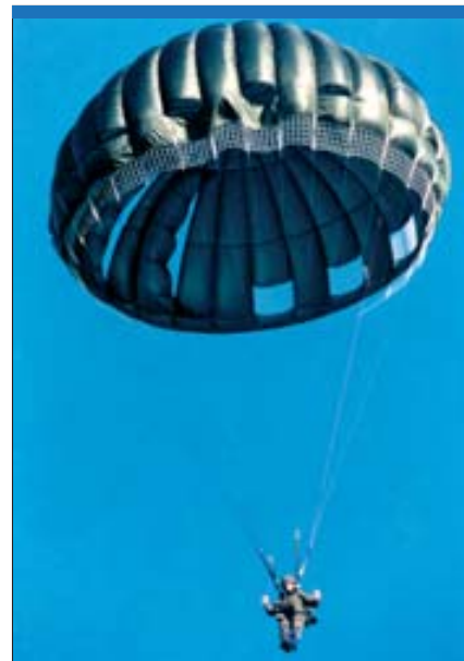
Socom is fielding the Airborne Systems MC-6 Special Operations Forces Tactical Assault Parachute System which provides units with a steerable parachute. (Airborne Systems)
