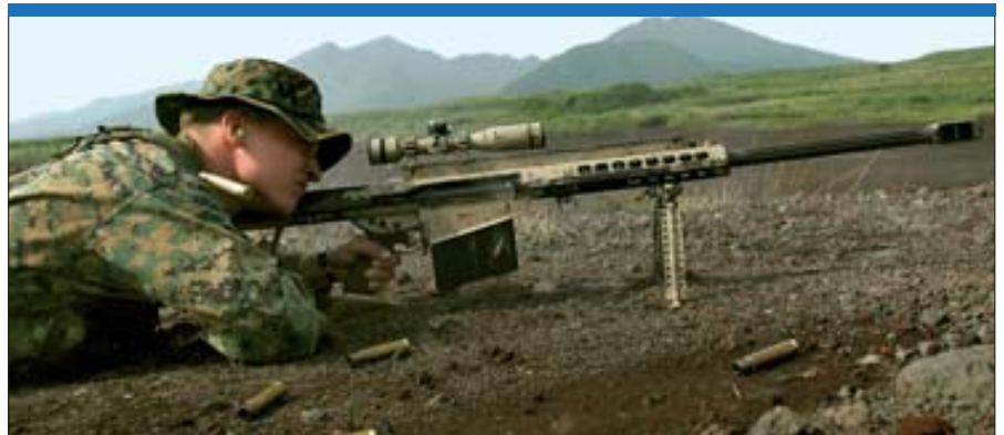
A US Marine Corps scout sniper team leader practises with the Barrett Firearms .50 calibre M82A3 Special Application Scoped Rifle. The weapon is widely employed in the EOD and anti-materiel roles. (US Marine Corps)
