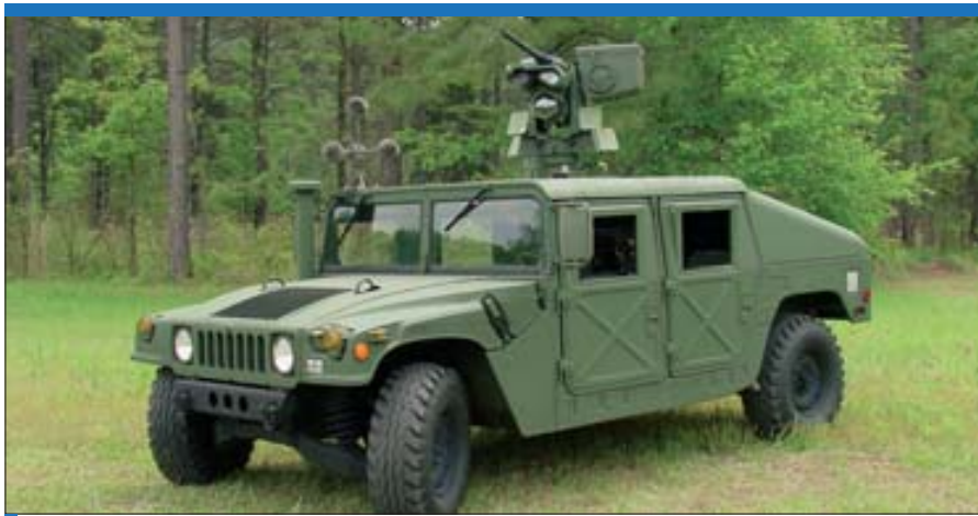
01dB-Metravib has supplied the Pilarw acoustic vehicle-mounted gunfire detection system for US Army special forces vehicles (seen here mounted above the right-hand windscreen of a Hummer) and for use in static facilities. (01dB-Metravib)
