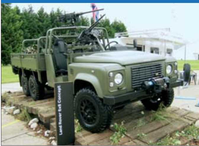
Land Rover has developed a 6 x 6 prototype vehicle that combines the all-terrain capability of its 4 x 4 light utility vehicles with greater payload. (Land Rover)
