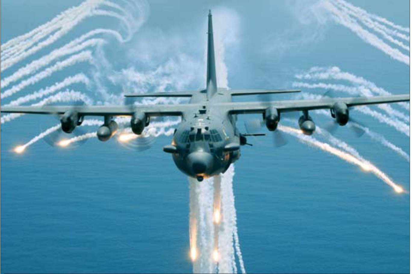
Flares are dispensed from a Lockheed Martin AC-130H Spectre of the 16th Special Operations Squadron, based at Hurlburt Field, Florida and forming part of the 1st Special Operations Wing. (US Air Force)
