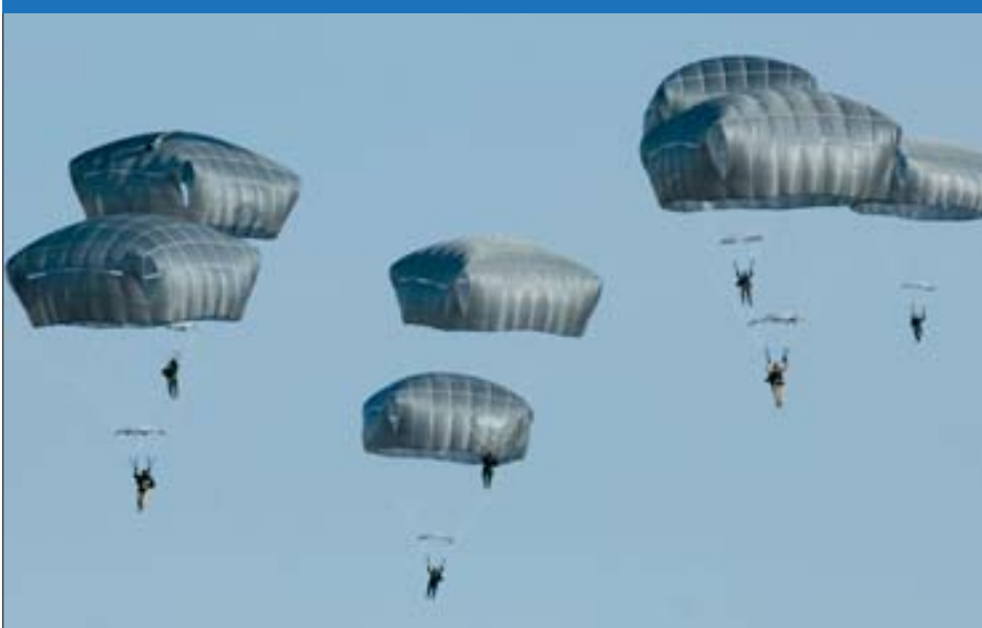
Scheduled to enter US Army service in 2008 the Airborne Systems T-11 Advanced Tactical Parachute System allows soldiers to make more controlled landings thus significantly reduce injuries during parachute operations. (Airborne Systems)
