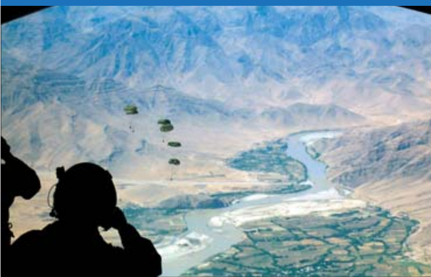
The US Air Force/Army Joint Precision Airdrop System (Jpads) is seen here under test in Afghanistan from Boeing C-17s of the 816th Expeditionary Airlift Squadron of the 379th Air Expeditionary Wing. (US Air Force)
