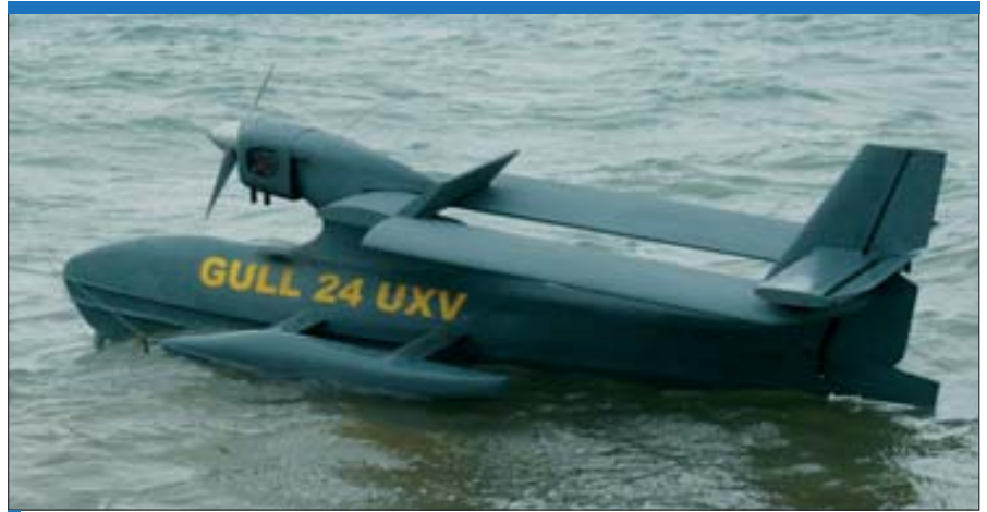
The Warrior (Aero Marine) Gull 24 is a technology demonstrator for the 70 kg Gull 36 amphibious drone, which is to be used in trials of formation operations off the Welsh coastline. (Warrior/Aero Marine)
