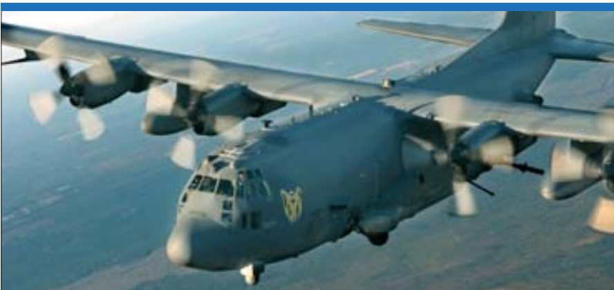
The AC-130U gun installation consists of a 25 mm General Dynamics GAU-12/U just ahead of the black sensor turret, a 40 mm Bofors further aft and a 105 mm howitzer at the rear. (Afsoc)
