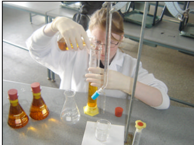
Titrating to find Biochemical Oxygen Demand of sea water.
