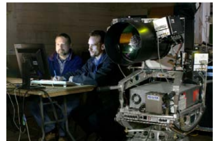
DRDC Defence Scientist Dean Haslip and a BTI employee using the Standoff Radiation Detector at night to detect radiation sources at a distance, during an exercise.
