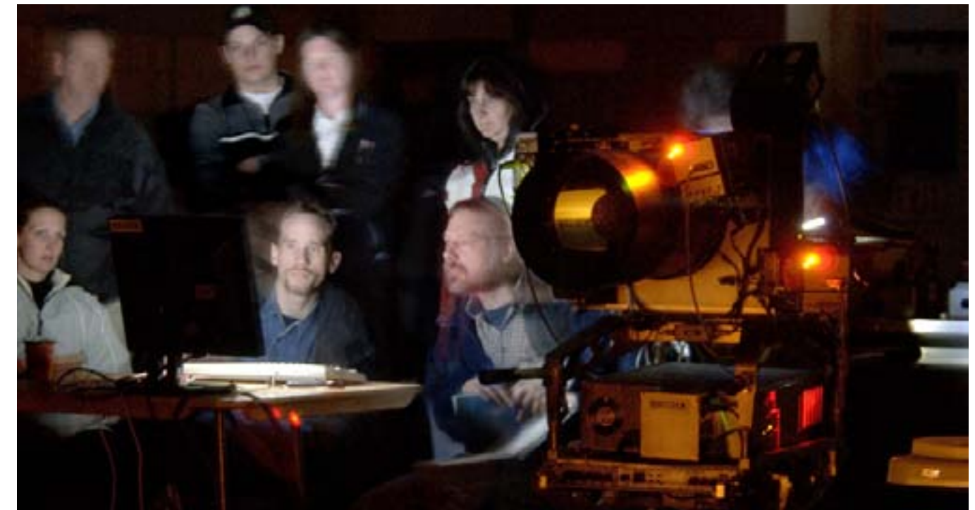
DRDC Defence Scientist Dean Haslip and a BTI employee (seated, right) using the Standoff Radiation Detector at night to detect radiation sources at a distance during an exercise. Other exercise participants observe results on the monitor.
