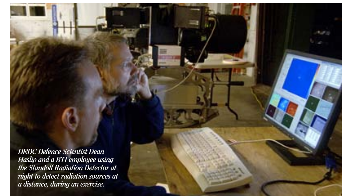
DRDC Defence Scientist Dean Haslip and a BTI employee (seated, right) using the Standoff Radiation Detector at night to detect radiation sources at a distance during an exercise. Other exercise participants observe results on the monitor.
