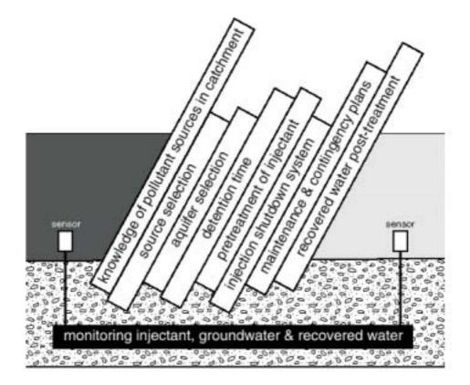
Figure 2 Multiple barriers to protect groundwater and recovered water at ASR projects (diagram CSIRO Land & Water)
