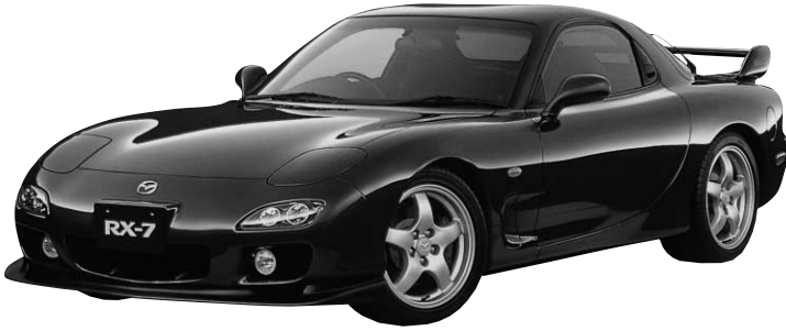
Face-lifted in late 1998, the Mazda RX-7 has a new front fascia with enlarged air intake areas for enhanced cooling efficiency.
