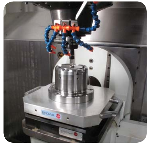
Bearing cell 5-axis machining center at Euclid facility
