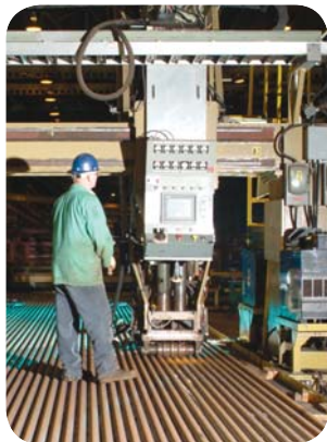
Wall panel membrane fabrication
