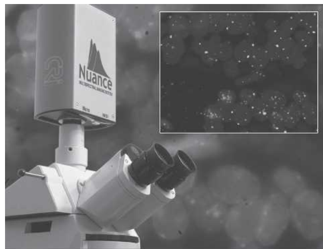
Figure 2 Nuance™ multispectral imaging system for microscopy. A spectral imaging camera similar to that inside the Maestro imager that mounts on any C-mount-equipped microscope (e.g., upright, inverted, or dissecting) provides multispectral imaging at the cellular and subcellular scale. The background and inset images illustrate a “before-and-after” example of the application of spectral unmixing to a fluorescence in situ hybridization (FISH) analysis of a breast cancer biopsy, separating tissue autofluorescence from fluorescently labeled nuclei, and Her2 and chromosome-17 molecular signals.
