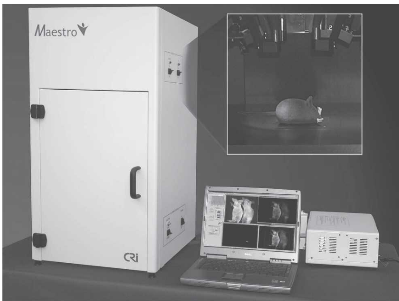
Figure 1 Maestro™ in vivo imaging system. An LCTF-based multispectral camera system and excitation source can capture reflectance and fluorescence images of small animals at multiple wavelengths. Spectral analysis software can then “unmix” multiple signals, removing autofluorescence contributions and increasing sensitivity and quantitative accuracy.
