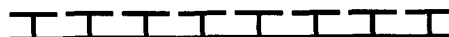
Figure 1 Cross-sectional view of a high-impedance, textured metal ground plane, consisting of metal protrusions on a flat conducting surface.
