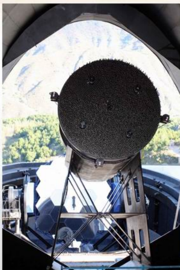
▲ 焦面板和光纤定位单元 The focal plane and fiber positioning units
