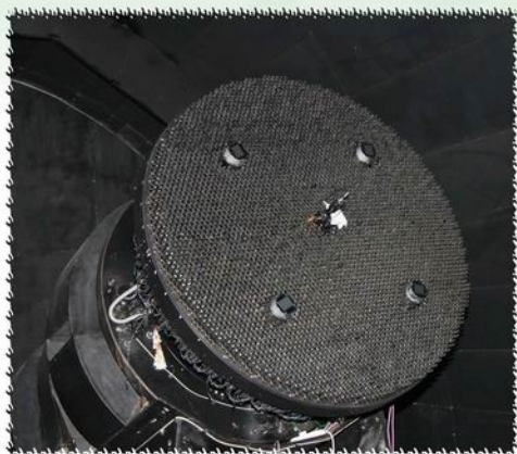
焦面板及4000个光纤定位单元 The focal plane with 4000 fiber positioning units
