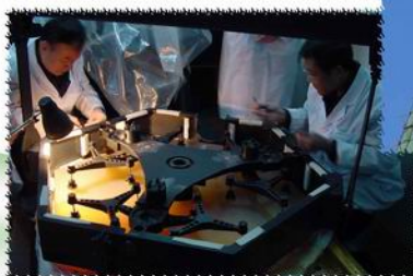
M_B 桁架吊装 Gross mirror cell of M_B during installation
