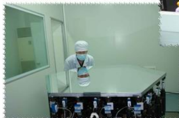
M_A 子镜及其支撑系统 M_A Sub-mirror and its support system
