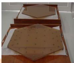
M A 子镜（薄镜面）及表面误差等高图 The M A thin sub-mirrors and its surface contour map
