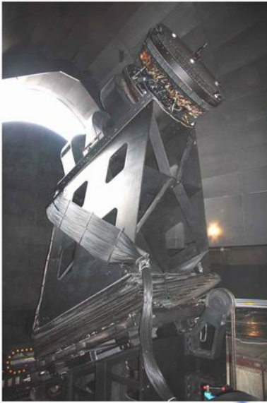
焦面机架 Mounting and tracking mechanism of the focal plate
