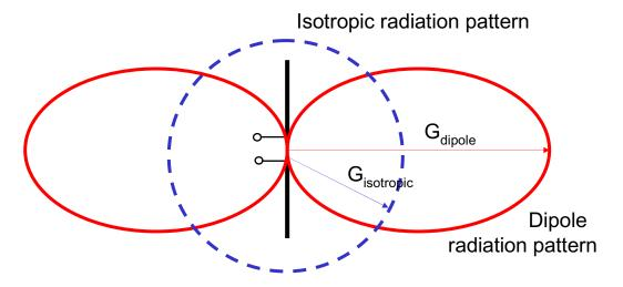
Real antennas such as dipoles, do not radiate uniformly in all directions (e.g. no power is radiated along the axis).
