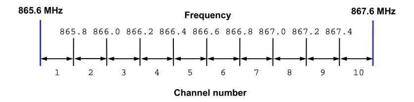
■ 10 channels of 200 kHz @ 2W ERP (3.2W EIRP)
