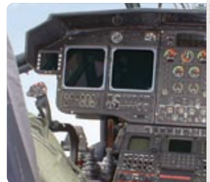
RNLAf AS-532 Cougar cockpit with Tactical Threat Display and Electronic Warfare Management System.
