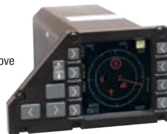
The Advanced Threat Display in semi-triangular version for the F-16.
