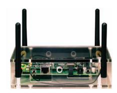
Quantenna's new QAC2300-RDK reference design includes schematics, layout, and design guidelines. The reference design enables rapid time to market with 2 Gbps dual-band, dual-concurrent operation (5 GHz 802.11ac plus 2.4 GHz 802.11n) using PCI-e or dual RGMII interfaces.
