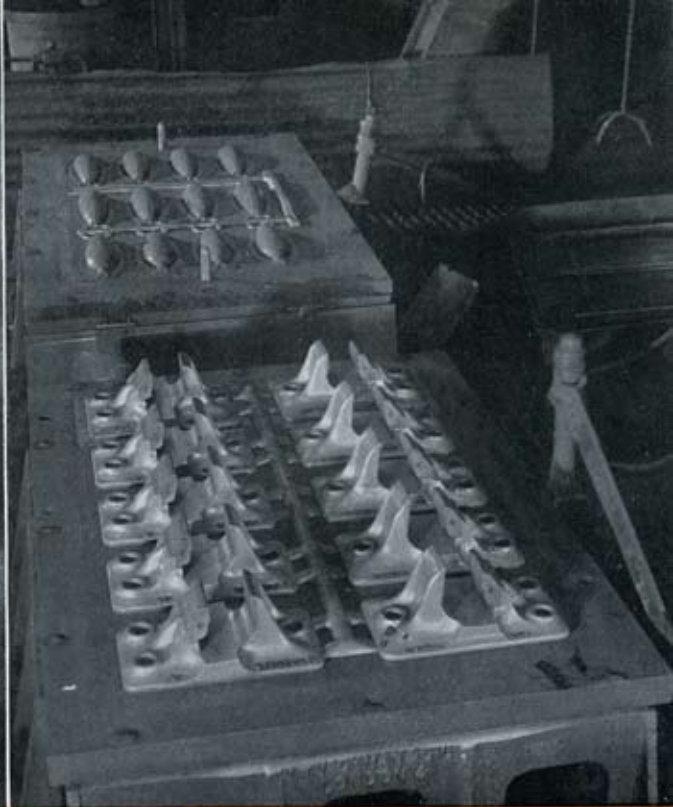
PATTERNS FOR RAILWAY CHAIRS AND TRENCH MORTAR BOMBS
