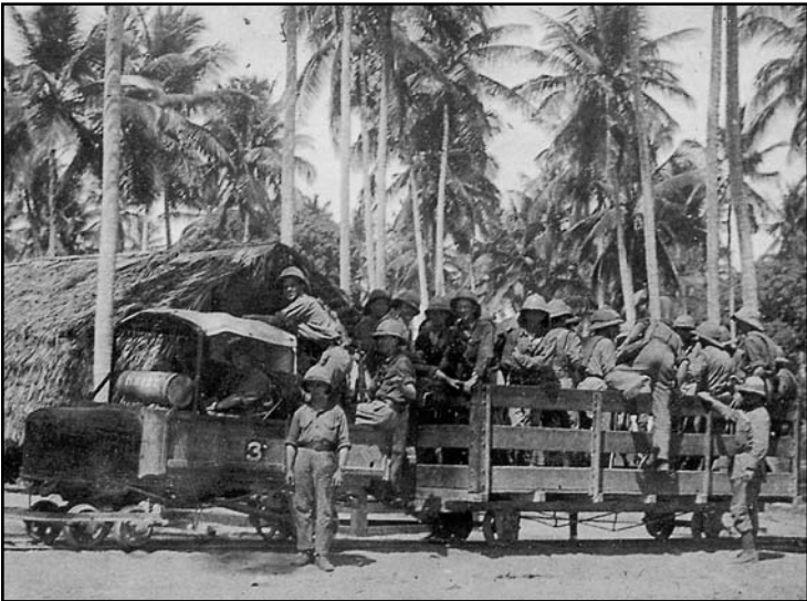
Bottom photograph shows 'motor lorry converted to tractor for service on railway' (see opposite).
