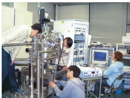
Experimental research on electronic states of thin films by angle-resolved ultraviolet photoelectron spectroscopy
