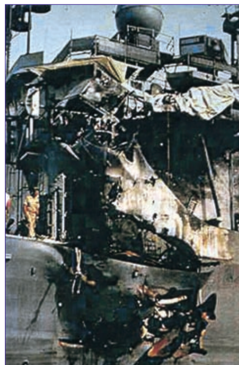
Missile damage to USS STARK FFG-31. The STARK is a similar vessel to the six RAN frigates. It was hit by two Exocet missiles launched by Iraqi forces in the Persian Gulf in 1987.
