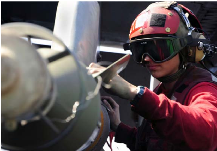
U.S. Navy Aviation Ordnanceman 2nd Class Marie Fentress affixes a GBU-12 laser-guided bomb to the wing of an F/A-18A+ Hornet aircraft on the flight deck of aircraft carrier USS Theodore Roosevelt (CVN 71), under way in the Pacific Ocean. The ship and embarked Carrier Air Wing (CVW) 8 are operating in the U.S. 5th Fleet area of responsibility.
