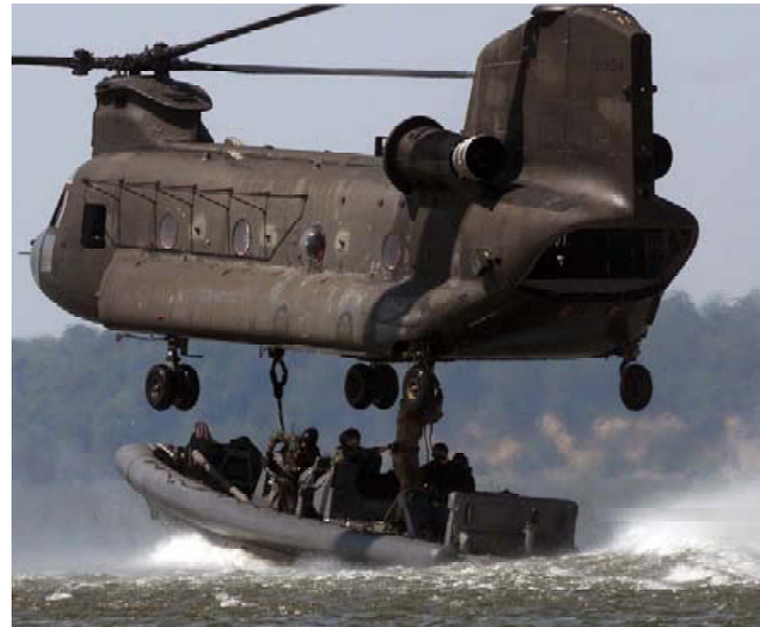
U.S. Navy Special Warfare Combatant-craft Crewmen (SWCC) assigned to Special Boat Teams 12 and 20 rig their rigid-hull inflatable boat to a CH-47 Chinook helicopter assigned to the 159th Aviation Regiment during a maritime external air transportation system (MEATS) training exercise in the Virginia Capes near Fort Eustis, Virginia. MEATS trains members of SWCC on extending their operational reach by attaching special operations crafts to helicopters for transport to remote locations for further training.
