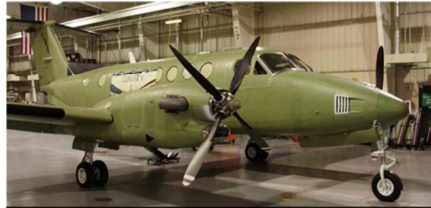
The first of thirty new King Air 350ERs was delivered to the USAF. The Air Force is rapidly configuring these aircraft with ISR equipment and redesignating them as MC-12W Liberty Aircraft. The initial MC-12W will arrive in theater in May 2009 and will provide critically needed multi-intelligence collection and targeting capabilities.
