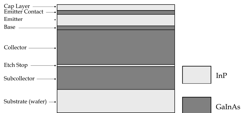
Figure 2.8: Layer structure on wafer as grown by MOMBE system
