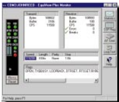
Monitor individual modems — busy them out, reset them and run loopback tests — while your system is running.
