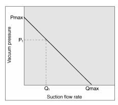
Flow characteristics are expressed in ejector vacuum pressure and suction flow. Flucuations in the suction flow rate will change the vacuum pressure. Normally this relationship is expressed in ejector standard use. In graph, Pmax is according to catalog use. Changes in vacuum pressure are expressed in the order below.
