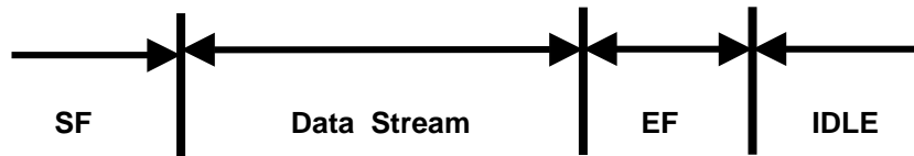
39 40 41 42 43 44 45 Figure 6.2 Frame Format
