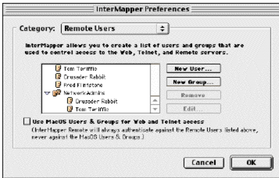
Figure 4-13a: Users and Groups may use the Classic MacOS or InterMapper's own Users and Groups list
