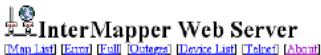
Figure 6-2: The header for the global web pages. Note that the navigational links list different choices from a map's links.
