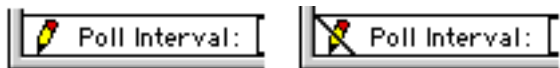
Figure 1-10: Monitoring mode indicators. The slash through the pencil indicates the map is not editable.
