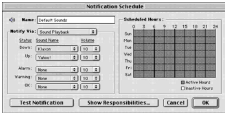
Figure 3-6: Schedule for Audible Alerts. A different sound may be assigned to denote the time a device goes into a new state (UP, DOWN, ALARM, etc.)
