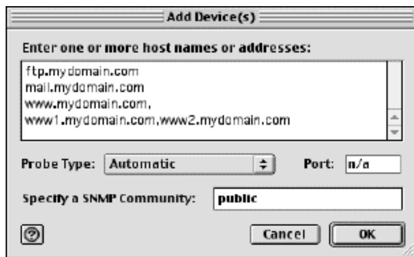
Figure 1-5: Add Device(s) window. Type or paste a list of DNS or AppleTalk NBP names or IP or AppleTalk addresses into this window. After you click OK, the items will be added to the map.
