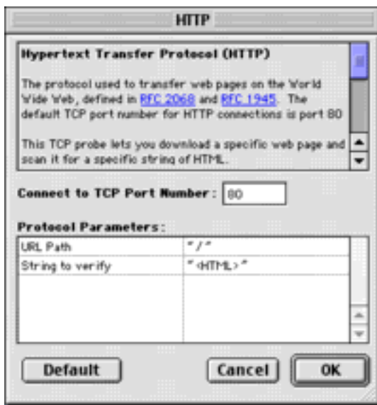
Figure 5-4: The Probe configuration window. This example shows the HTTP probe which has parameters for the remote port, the URL Path and the string that is expected in the response.
