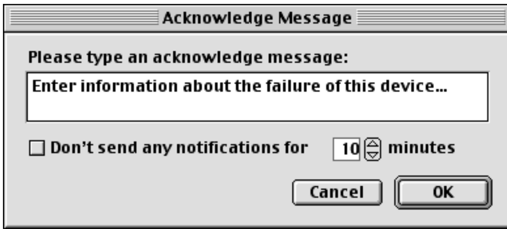
Figure 2-16: The Acknowledge Message Window. Data typed here will be entered into the InterMapper log file as well. Checking the Don't send notifications... box will hold off notifications for the specified number of minutes.
