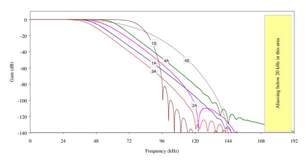
Symmetric (S) and Asymmetric (A) ADC Filters Used - Frequency Responses Fs is 192 kS/s
