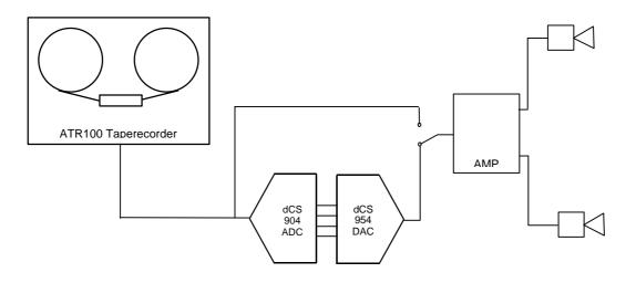
Figure 1 – High Sample Rate Demonstration setup
