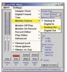
The Settings menu contains a surprising number of options including selections for 'zero'-latency monitoring, record and play dither, and well as advanced options for instrumentation purposes. switched into record mode, and there is no peak-hold indicator or readout, which would be very useful on the inputs. Beneath the meters are volume faders that can be ganged for stereo operation by ticking the 'Channel Lock' option in the Setting menu, and each channel pair also has a Mute button.
