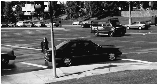
FIGURE 4 Primary hazard zones are those in which the pedestrians are hit while crossing on green. Secondary hazard zones are the crosswalk areas on the cross street.
