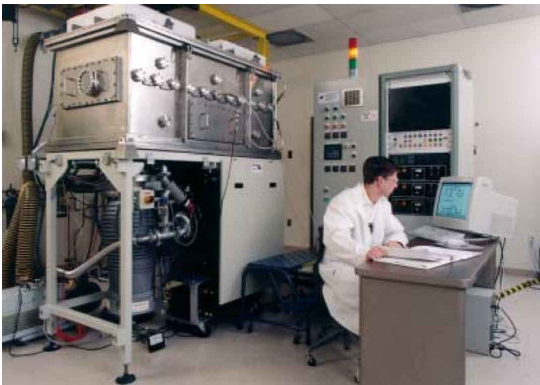
Figure 2.10 In-line CIGS deposition system.
