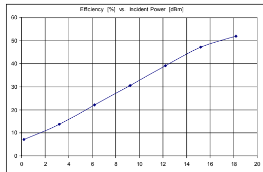
Figure 2. Efficiency measurements of a 10 GHz rectenna array with Schottky diodes wire-bonded at the feedpoints of the antenna. Efficiencies > 50 % are demonstrated for relatively large-area arrays (~ 20 cm) and are limited only by saturation of the diodes. Efficiencies approaching 90% are likely with better-quality diodes.
