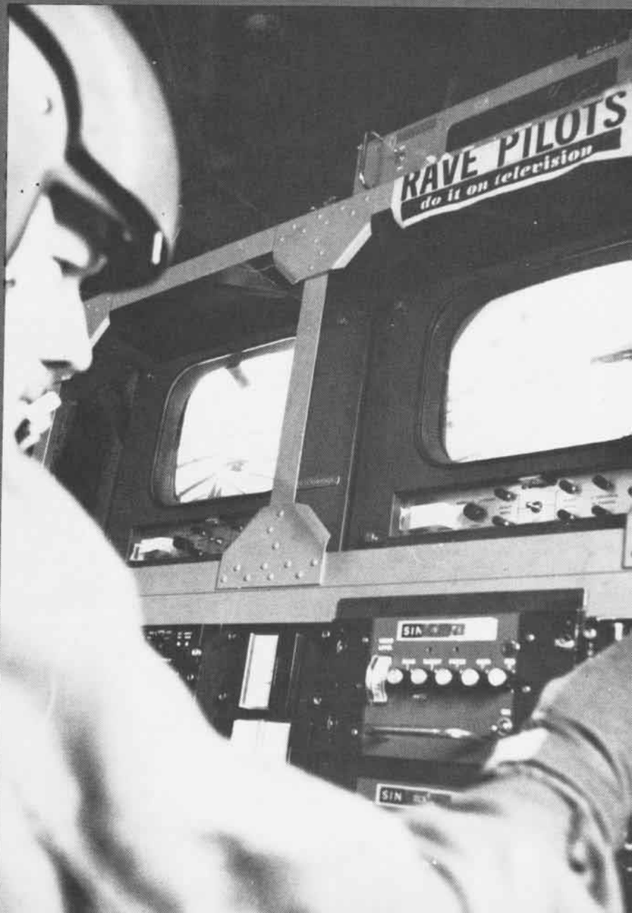
In flight control station, pilot's only visual references are three TV monitors, left. Below, engineer adjusts monitors, controls data collection and instructs subject pilot.
