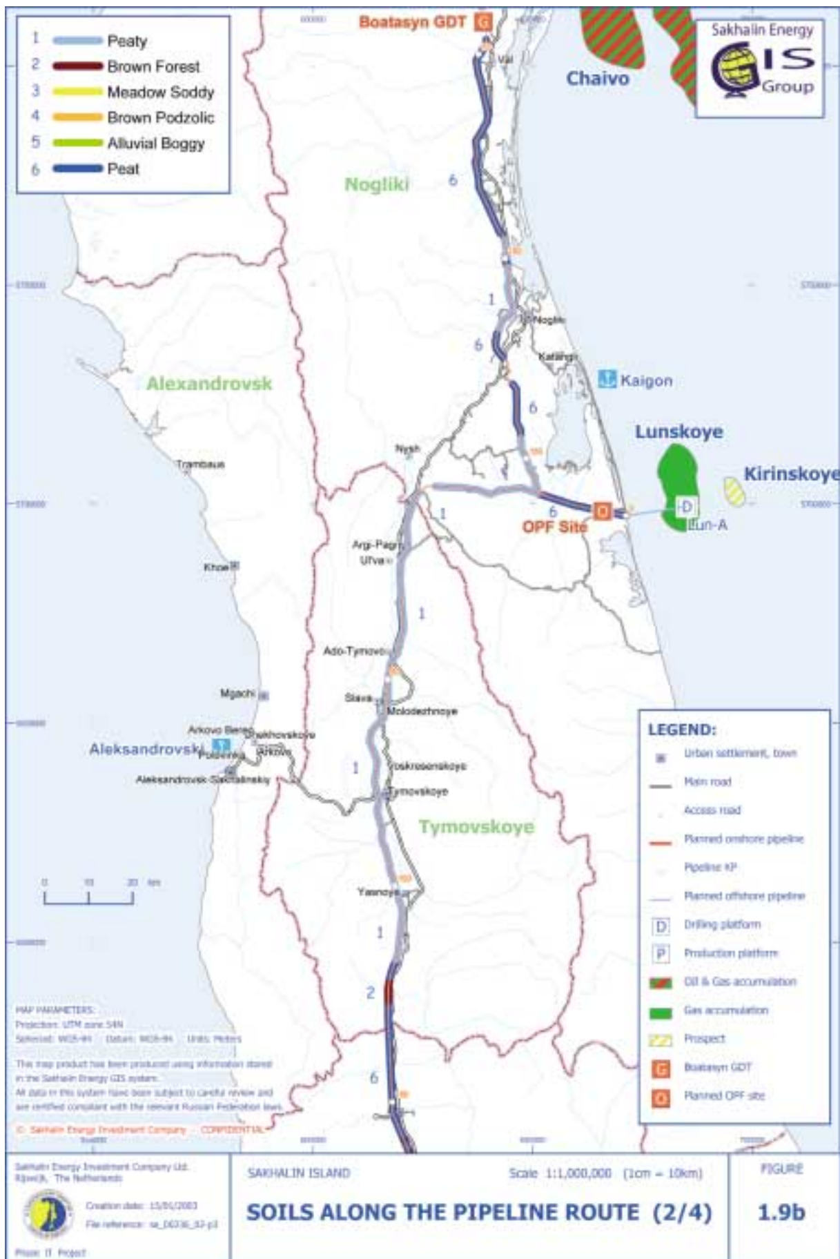
Figure 1.9b Soils Along the Pipeline Route
