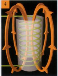
The FIELD is a hollow cylindrical casing that surrounds the coil. Since a magnetic flux path flows more easily through iron or steel, this tubular casing adds strength to the magnetic flow.
