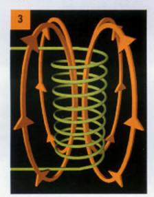
The COIL is comprised of many turns of tightly wound copper wire. When DC current flows through this wire, it creates a strong magnetic flux path which flows around the coil and through its center in a doughnut shape.
